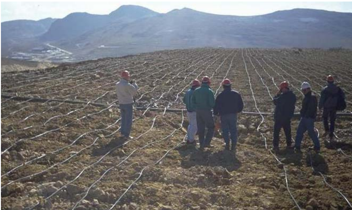
Figure 4. Drip-emitter recirculation of external barren solution onto ore heap top lift surface for controlled active leaching.
