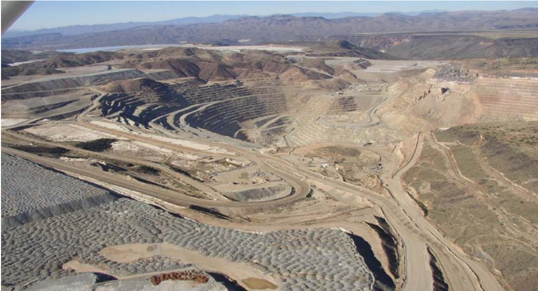
Figure 1 – Active open pit copper mine operation showing a mine waste (non-ore) rock pile in the foreground with a heap leach pad and tailings impoundment in the background surrounding a relatively steep walled open pit excavation.
