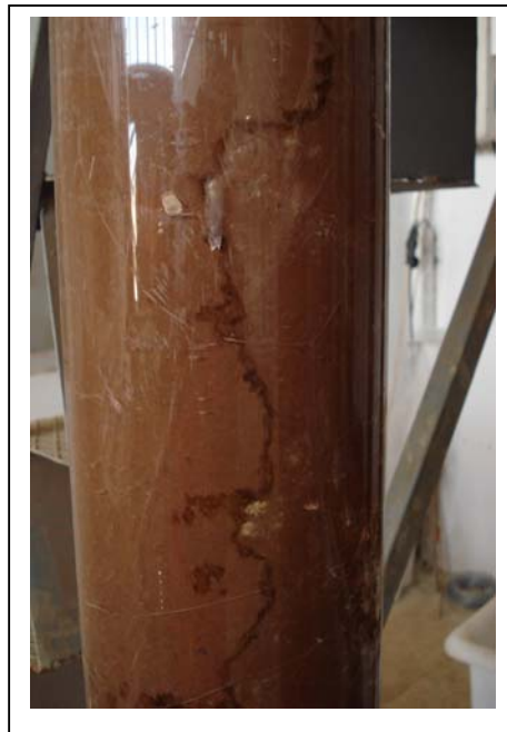
Figure 3.1 Channelling in a small diameter column
