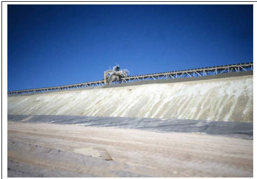
Figure 3.5 Tripper Stacker Operating in Advance Mode, Chile
