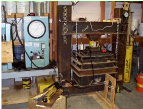
Photo 1: Pipe Deflection Test Apparatus
