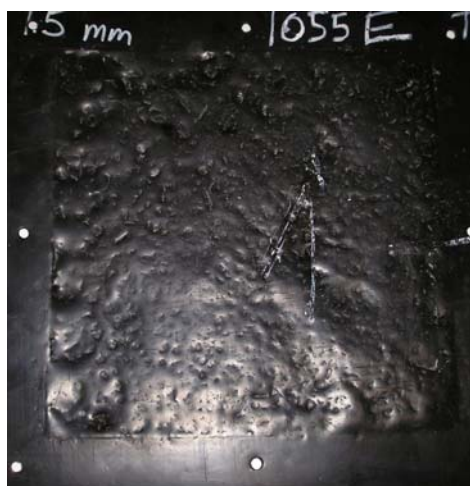
Figure 1. Puncture test specimen of 1.5mm LLDPE tested at 120m simulated heap height and temperatures of ambient (left) and 60°C (right). White circles (right) show points of significant thinning and eminent penetration.
