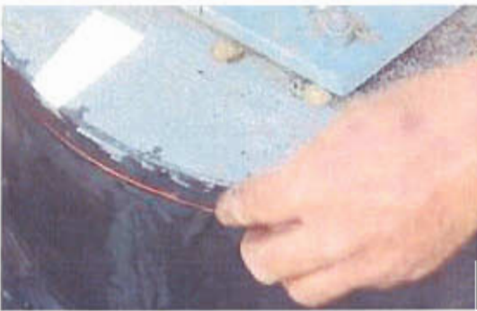
(e) Embedding copper wire before weld for spark test.
