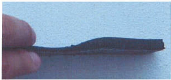
(f) Gasket that was under an overlapped batten showing a section that was crushed past its elastic limit, and a section that was not compressed.
