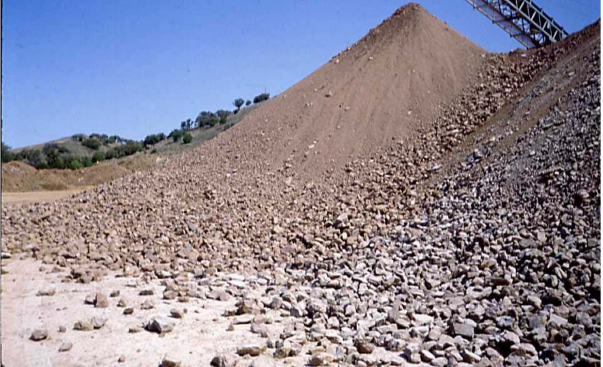
Photo 1 – Segregated Earthfill at Top and Rockfill at Bottom of Ore Stockpile
