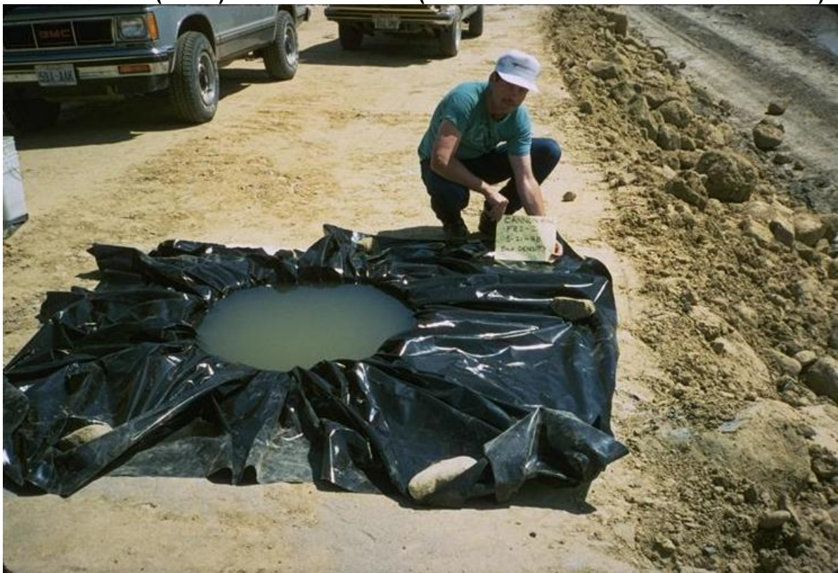
PHOTO 9 – PREPARATION FOR ROCKFILL DENSITY AND GRADATION TEST USING A 3 FT (0.9 M) DIAMETER RING (NOTE OVERSIZED ROCK ON SLOPE)
