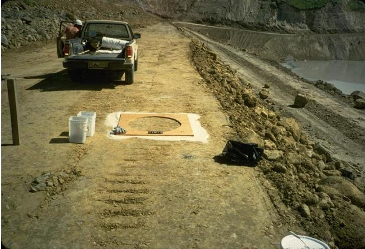
PHOTO 9 – PREPARATION FOR ROCKFILL DENSITY AND GRADATION TEST USING A 3 FT (0.9 M) DIAMETER RING (NOTE OVERSIZED ROCK ON SLOPE)
