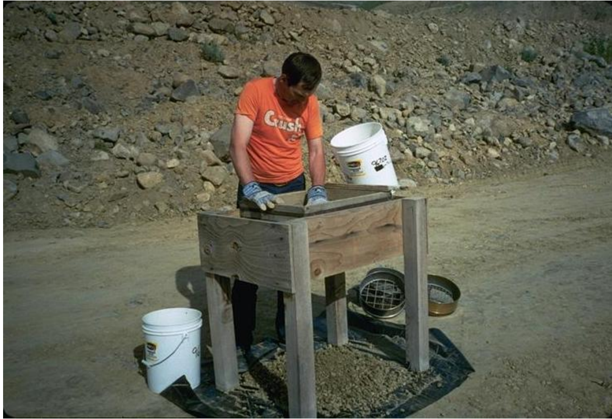
PHOTO 11 – SEPARATION OF MINUS ¾ INCH (19 MM) SQUARE MESH SOIL PARTICLES FROM LARGER GRAVEL AND COBBLE SIZED ROCK FRAGMENTS
