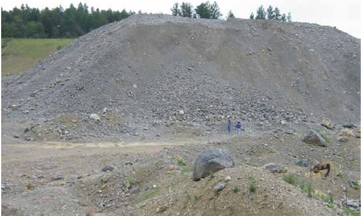
PHOTO 1 – ROCKFILL BORROW STOCKPILE WITH SOME ROCK SEGREGATION SHOWN ON EXTERIOR SLOPES
