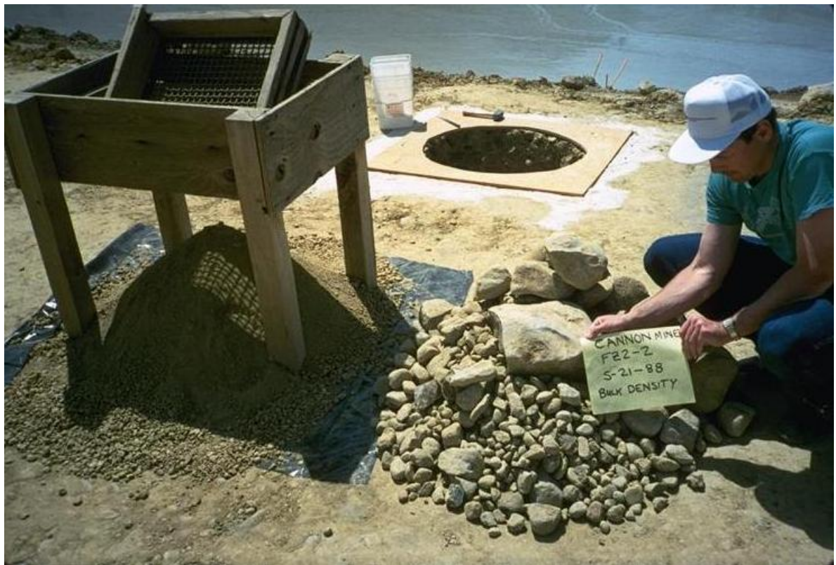
PHOTO 11 – SEPARATION OF MINUS ¾ INCH (19 MM) SQUARE MESH SOIL PARTICLES FROM LARGER GRAVEL AND COBBLE SIZED ROCK FRAGMENTS
