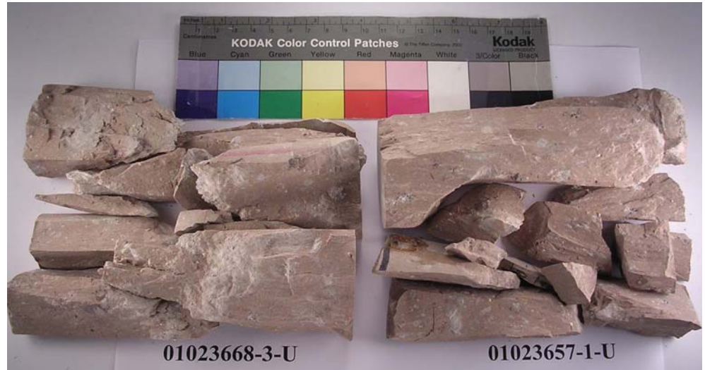
Fig. 2 Specimens after failure. Longitudinal splitting dominates the failure mode. Vapor-phase altered ( white ) spots are present inside the specimens: 01023668-3-U (strain rate = 1.36 \times 10^{-8} \text{ s}^{-1} ) and 01023657-1-U (strain rate = 1.13 \times 10^{-5} \text{ s}^{-1} )
