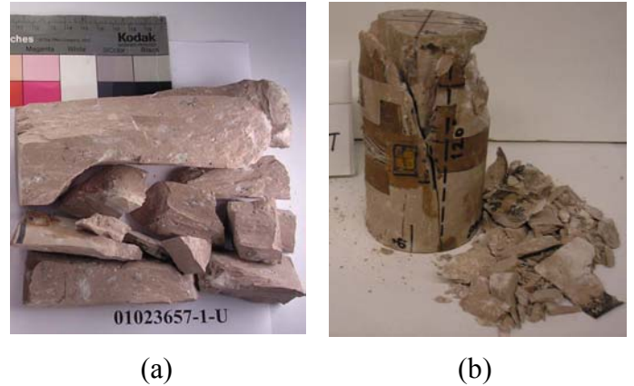
Fig. 6. Specimens after failure: (a) After uniaxial test, longitudinal splitting dominates the failure mode. Specimen ID: 01023657-1-U (stress rate = 0.3805 MPa/s); (b) After triaxial test, shear failure. Specimen ID: 01026241-1-T (stress rate = 0.0035 MPa/s, confining pressure = 5 MPa).
