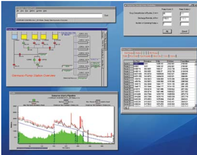
Above Typical Pipeline Simulator monitor screen
