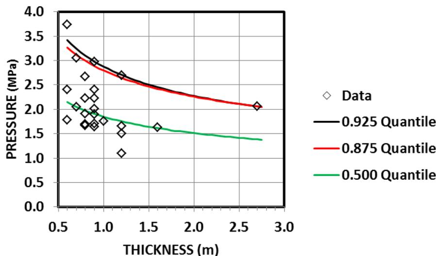
Figure 6 : Single Medof Panel Column Data and Quantile Regression
