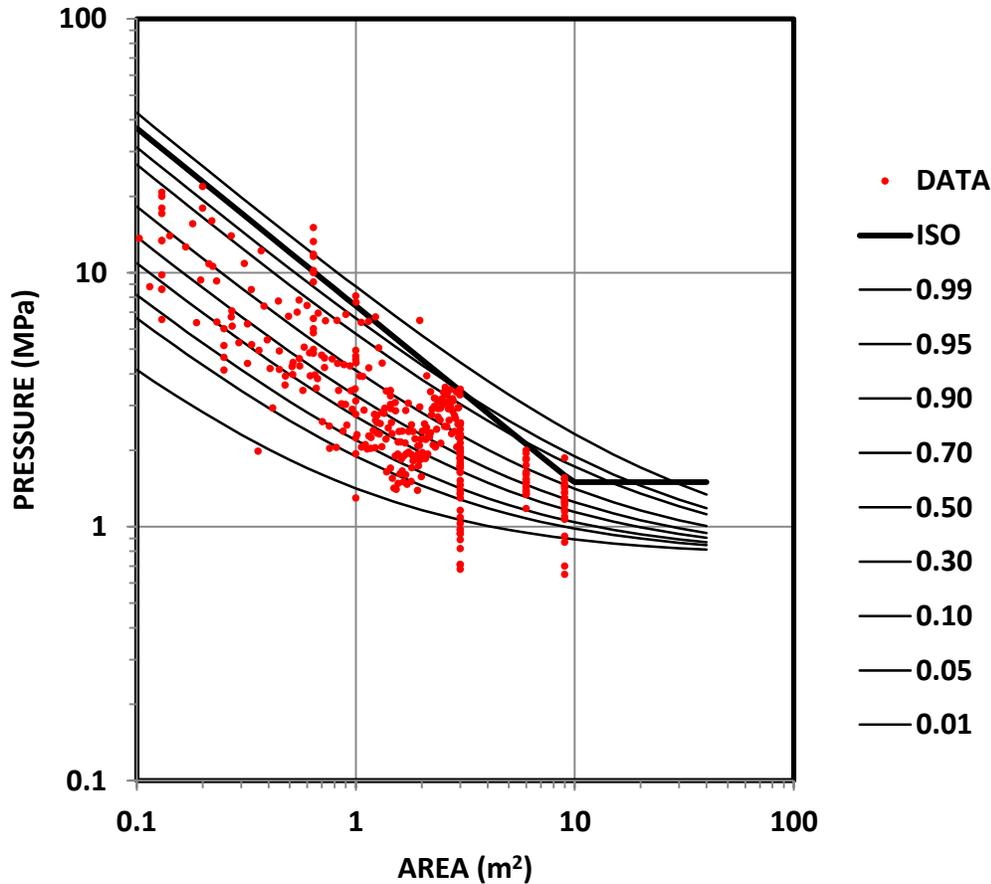
**Figure 2 : Quantile Regressions Fitted to:  $\text{Pressure} = \text{Multiplier} \times \text{Area}^{-0.716} + 0.766 \text{ MPa}$ ; Local Pressure**
