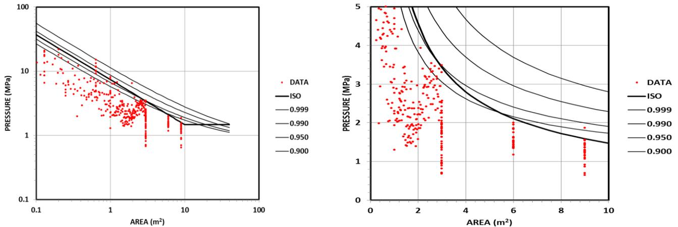
**Figure 4 : Local Pressure Design Values at Various Quantiles (Log Plot - left and Linear Plot - right)**
