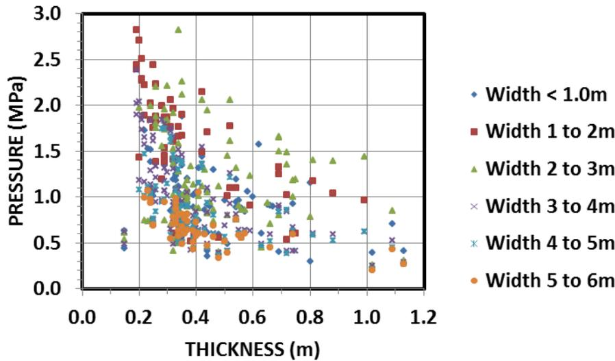
Figure 10 : Pressure Data from Multiple Panels for various interaction widths and thickness; Baltic Data
