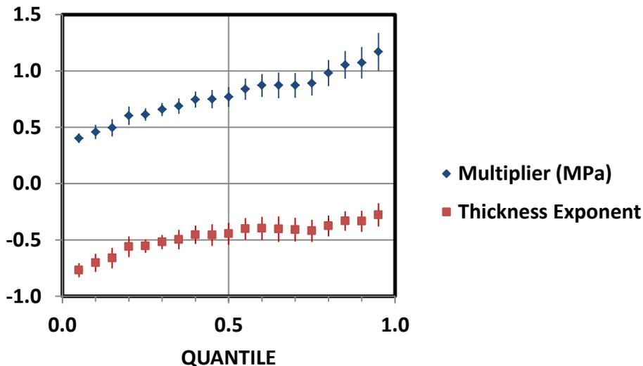
Figure 9 : Values of Fitted Parameters from Quantile Regression to Power Law on Thickness; Single Panel Baltic Data
