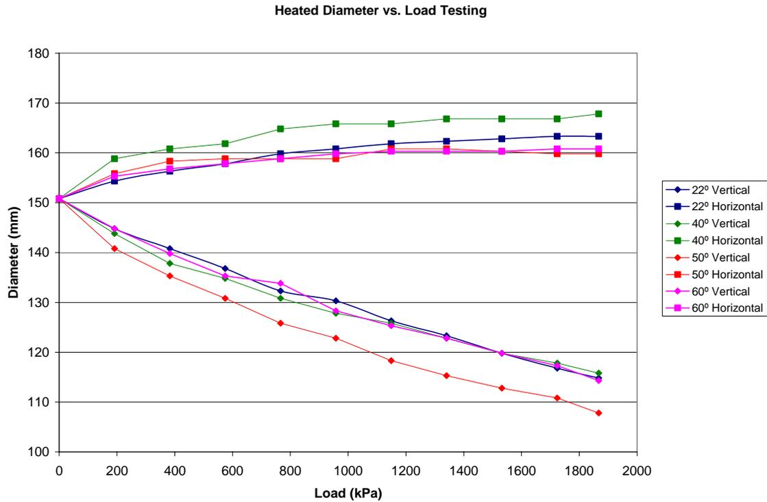
Figure 2 - Pipe Loadings and Varying Temperatures
