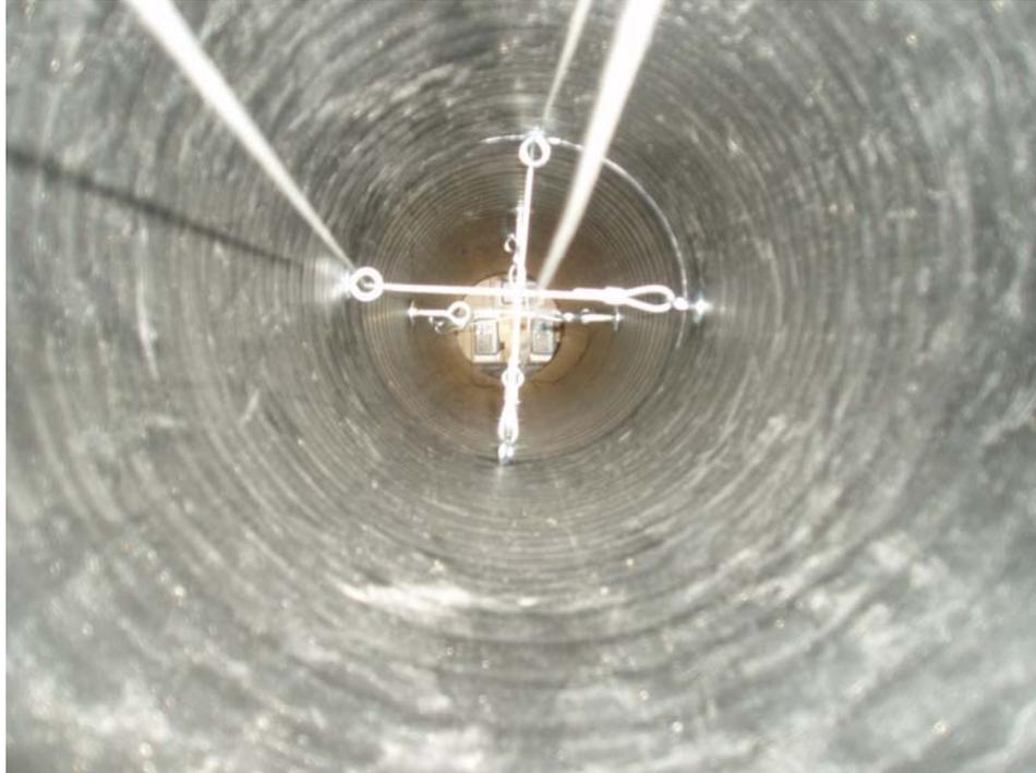
Photo 2 - Deflection Measurement System Before Test
