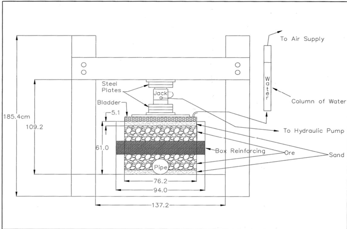
Figure 1 - Test Apparatus
