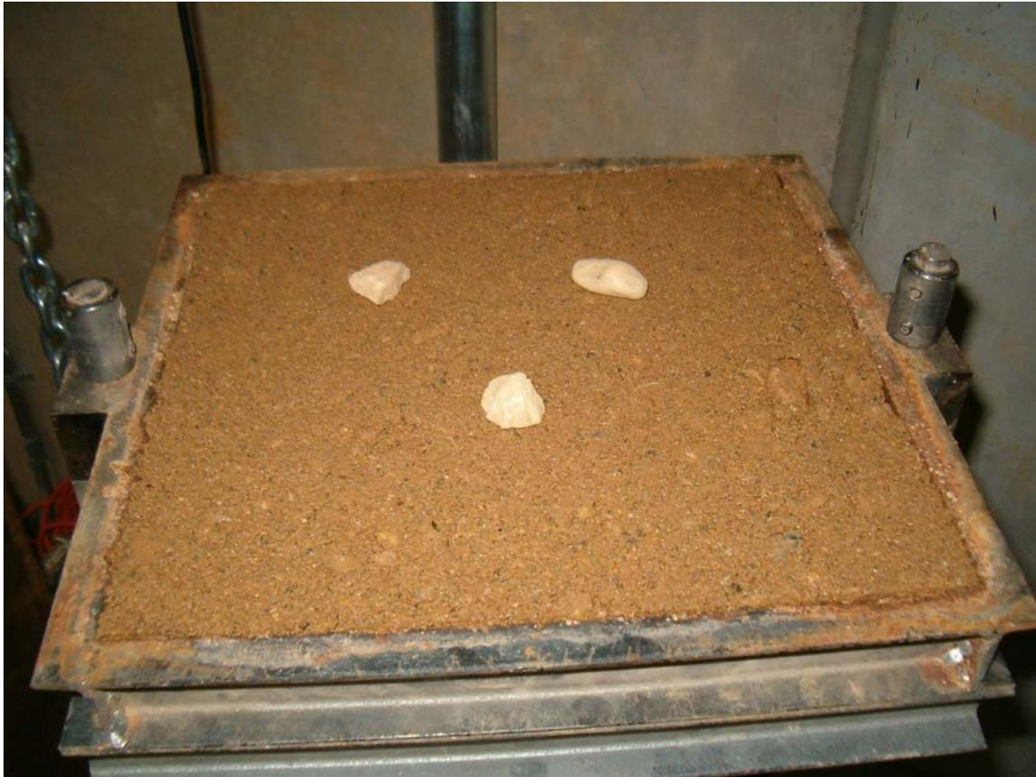
Figure 3. 40-mil geomembrane sample results
