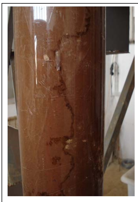
Figure 3.1 Channelling in a small diameter column
