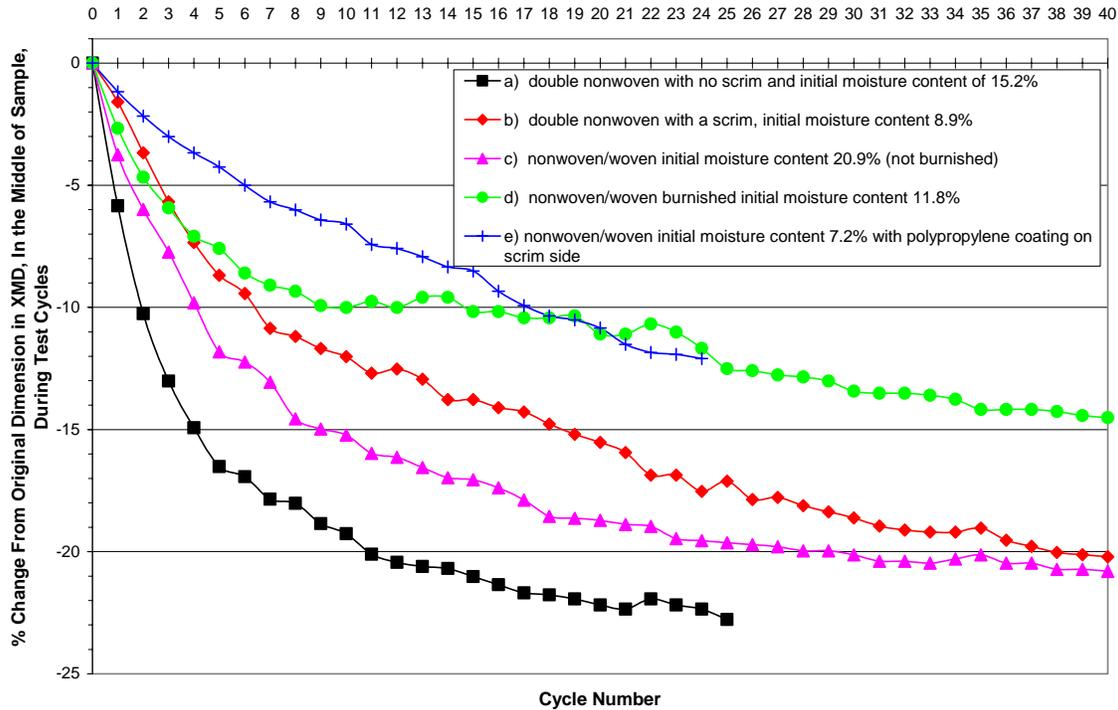
Cyclic wetting and drying can be caused by the diurnal temperature swings, which can be very large under a geomembrane. Daytime temperatures can reach 60 or 70°C on black geomembrane, while night time temperatures will be about ambient. This will cause cyclic vapor/condensate phases with a resulting cyclic change in water content in the GCL. Longer-term, the GCL can exchange water with the subgrade, depending on their relative matric-suction properties.
