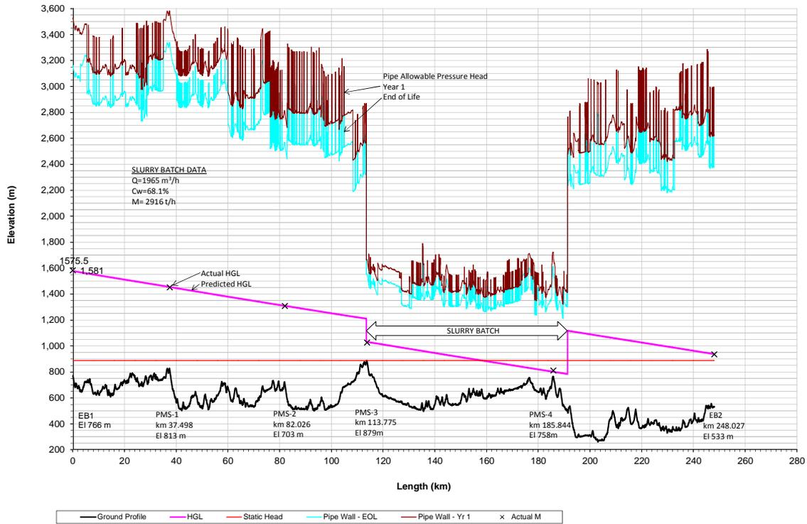
Figure 5 Section 1 Hydraulics EB1 to EB2 (Batch 04-2015)
