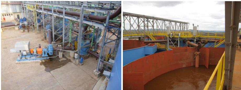
Figure 4 Charge pumps and agitated tanks
