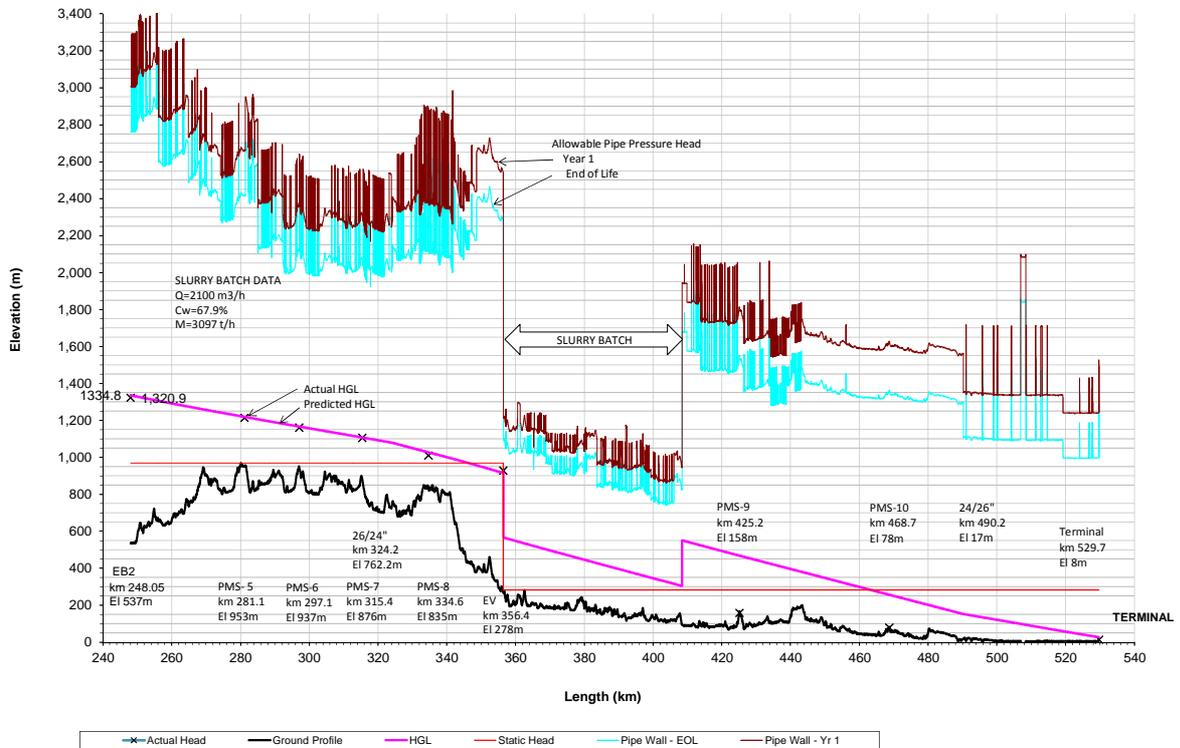
Figure 6 Section 2 Hydraulics EB2 to Terminal (Batch 07-2014)
