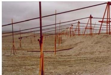
Fig. 2: Hydro-cyclone towers for underflow tailings beach development
