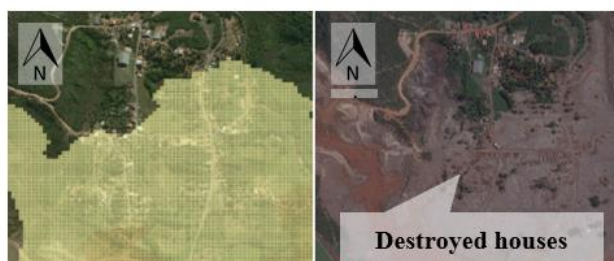
Figure 4 Bento Rodrigues flood prediction model (left side image) versus after-disaster situation (right side image)
